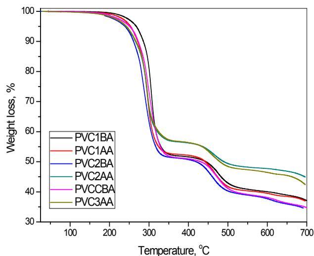
**Figure 4.** TGA Curve of PVC cable outer sheaths before and after 500 hrs UV ageing.
