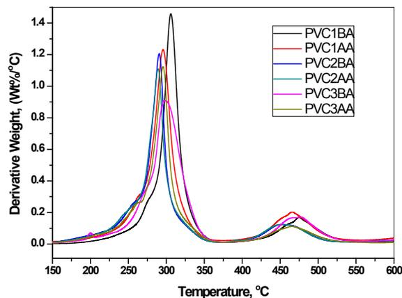
**Figure 5.** DTG Curve of PVC cable outer sheaths before and after 500 hrs UV ageing.
