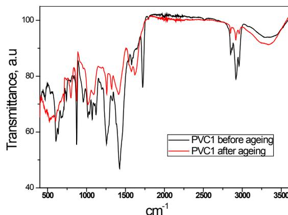
**Figure 6.** FTIR of PVC1 before and after 500 hrs UV ageing.
