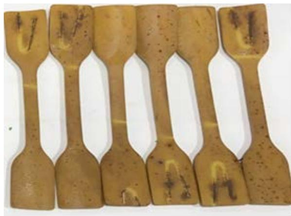
**Figure 3.** Colour change of PVC1 after 500 hrs UV ageing.
