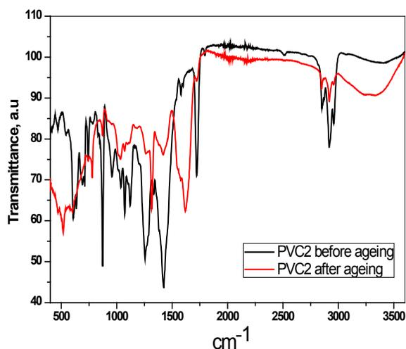
**Figure 7.** FTIR of PVC2 before and after 500 hrs UV ageing.
