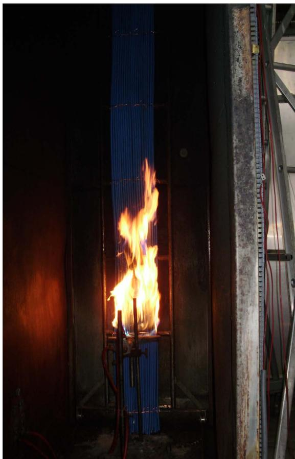
**Figure 1.** Flammability test on bunch of cables.
