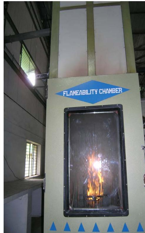
**Figure 2.** Flammability test chamber.
