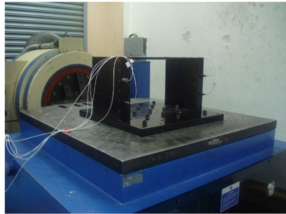
**Figure 1.** Typical fixture for relay mounting.
