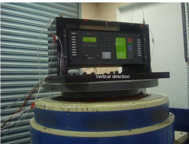
**Figure 2.** Relay test arrangement in three mutual perpendicular axes.
