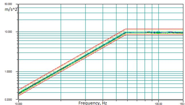
**Figure 4.** Vibration response test profile.
