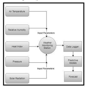
Figure 4. Simplified weather station signal-flow diagram.
