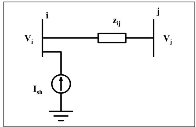
FIG. 1 CURRENT INJECTION MODEL OF SVC.
