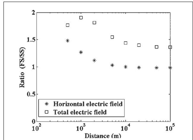
FIG. 6 RATIO OF FIRST TO SUBSEQUENT RETURN STROKE ELECTRIC FIELD PEAKS AS A FUNCTION OF RADIAL DISTANCE (FOR THE OBSERVATION POINTS AT A HEIGHT OF  $z = 10$  m), ABOVE THE GROUND PLANE OF WORST CASE FINITE GROUND CONDUCTIVITY ( $\Sigma_G = 0.0001$  S/M).
