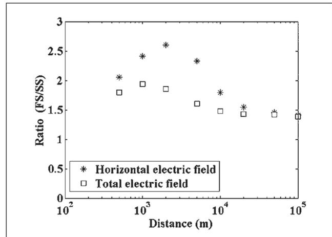
FIG. 4 RATIO OF FIRST TO SUBSEQUENT RETURN STROKE ELECTRIC FIELD PEAKS AS FUNCTION OF DISTANCE FOR THE OBSERVATION POINTS AT A HEIGHT OF  $Z=10$  m, ABOVE THE PERFECTLY CONDUCTING GROUND.
