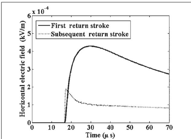
FIG. 3 HORIZONTAL COMPONENT OF ELECTRIC FIELD DUE TO FIRST AND SUBSEQUENT RETURN STROKE ABOVE THE PERFECTLY CONDUCTING GROUND AT  $Z=0$  m,  $R=5000$  m.
