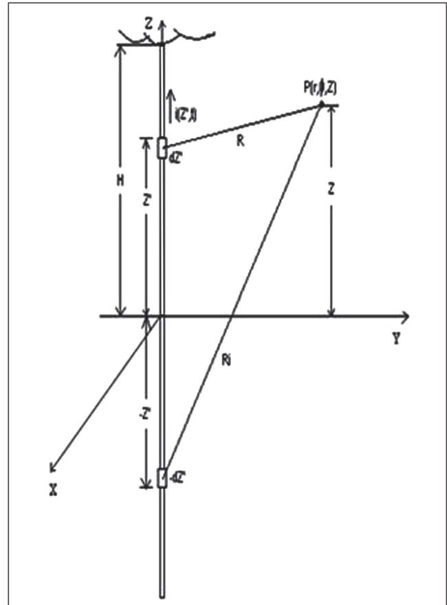
FIG. 1 GEOMETRICAL DETAILS OF LIGHTNING CHANNEL USED FOR LIGHTNING ELECTROMAGNETIC FIELD CALCULATIONS
