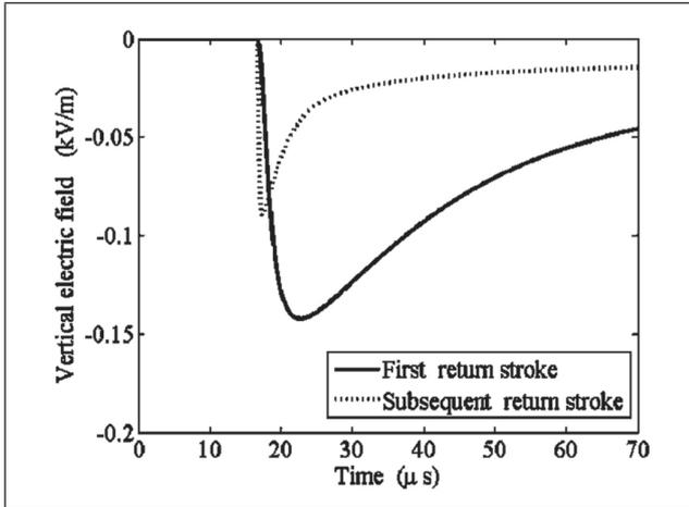
FIG. 2 VERTICAL COMPONENT OF ELECTRIC FIELD DUE TO FIRST AND SUBSEQUENT RETURN STROKE ABOVE THE PERFECTLY CONDUCTING GROUND AT  $Z=10$  m,  $R=5000$  m.
