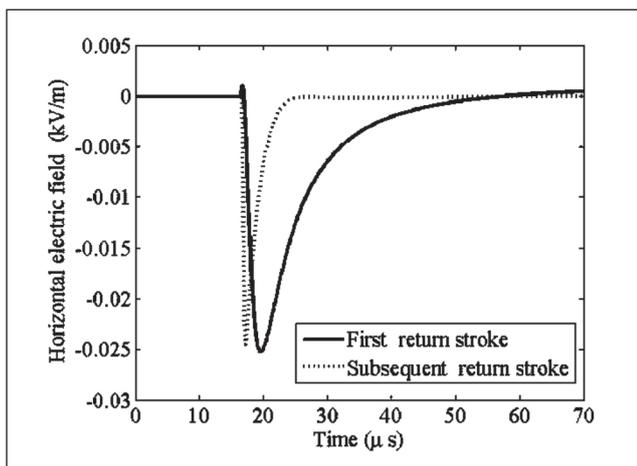
FIG. 5 HORIZONTAL ELECTRIC FIELD DUE TO FIRST AND SUBSEQUENT RETURN STROKE ABOVE GROUND AT  $z = 10$  m,  $r = 5000$  m FOR FINITELY ( $\Sigma_G = 0.0001$  S/M) CONDUCTING GROUND.
