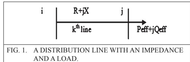
FIG. 1. A DISTRIBUTION LINE WITH AN IMPEDANCE AND A LOAD.
