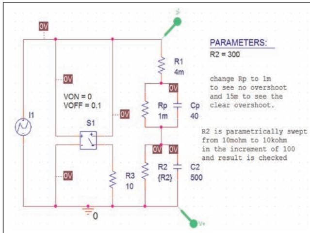
FIG. 4. PSPICE FUNDAMENTAL MODEL CIRCUIT OF HYBRID CAPACITOR MODULE (6 CAPACITORS IN SERIES) WITH LEAKAGE RESISTANCE PARAMETRIC SWEEP.
