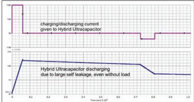
FIG. 6. SIMULATION RESULT OF FUNDAMENTAL CIRCUIT FOR VALUE OF R2 CHOSEN - 300  $\Omega$ .
