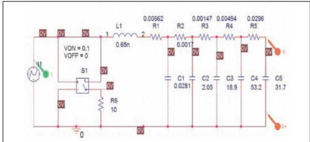
FIG. 8. 5TH ORDER LADDER EQUIVALENT CIRCUIT OF MAXWELL™ 100F IN PSPICE
