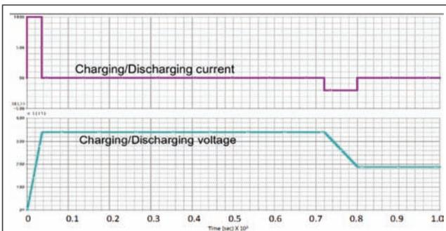
PSPICE models of the 5<sup>th</sup> order MAXWELL™ 100 F super capacitor is shown in Figure (s). 8
