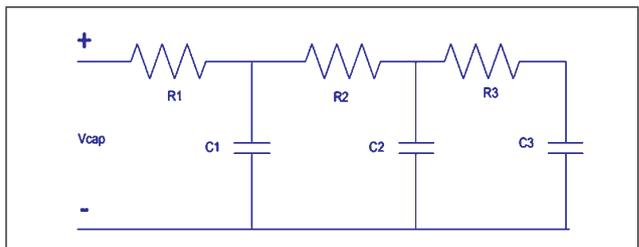
FIG. 7: 3RD ORDER RC LADDER NETWORK WITHOUT INDUCTANCE.
