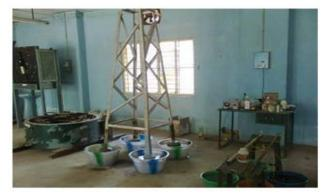
Figure 12. Model tower. (a). Coatings being applied (b). Corrosion test in progress.
