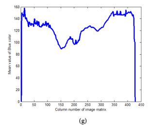
**Figure 4.** Analysis of Thermal Image for Bearing fault (defected Ball) of Induction Motor after 10 min. run ( side view). (a) Bearing fault (defected Ball) of Induction Motor after 5 min. run (side view). (b) Max value of Red colour. (c) Max value of Green Colour. (d) Max of Green Colour. (e) Mean of Red Colour. (f) Mean of Green Colour. (g) Mean of Blue colour.
