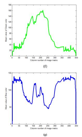
Figure 5. Thermal Image analysis of Healthy Induction Motor- front view. (a) Healthy Bearing of Induction Motor - front view. (b) Max value of Red colour. (c) Max value of Green colour. (d) Max value of Blue colour. (e) Mean value of Red colour. (f) Mean value of Green colour. (g) Mean value of Blue colour.
