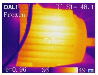
Figure 1. Thermal image of a running induction motor.
