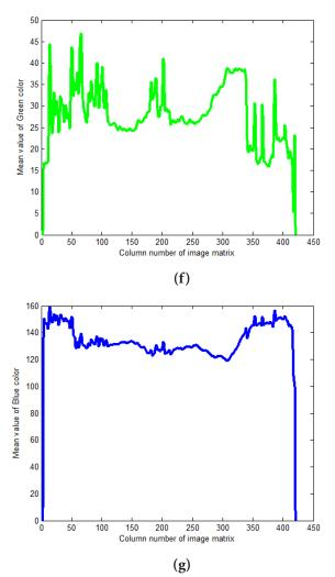
Figure 3. Analysis of Thermal Image of Healthy bearing Induction Motor (side view). (a) Thermal Image of Healthy bearing Induction Motor (side view). (b) Max value of Red colour. (c) Max value of Green colour. (d) Max value of Blue colour. (e) Mean value of Red colour. (f) Mean value of Green colour. (g) Mean Value of Blue colour.
