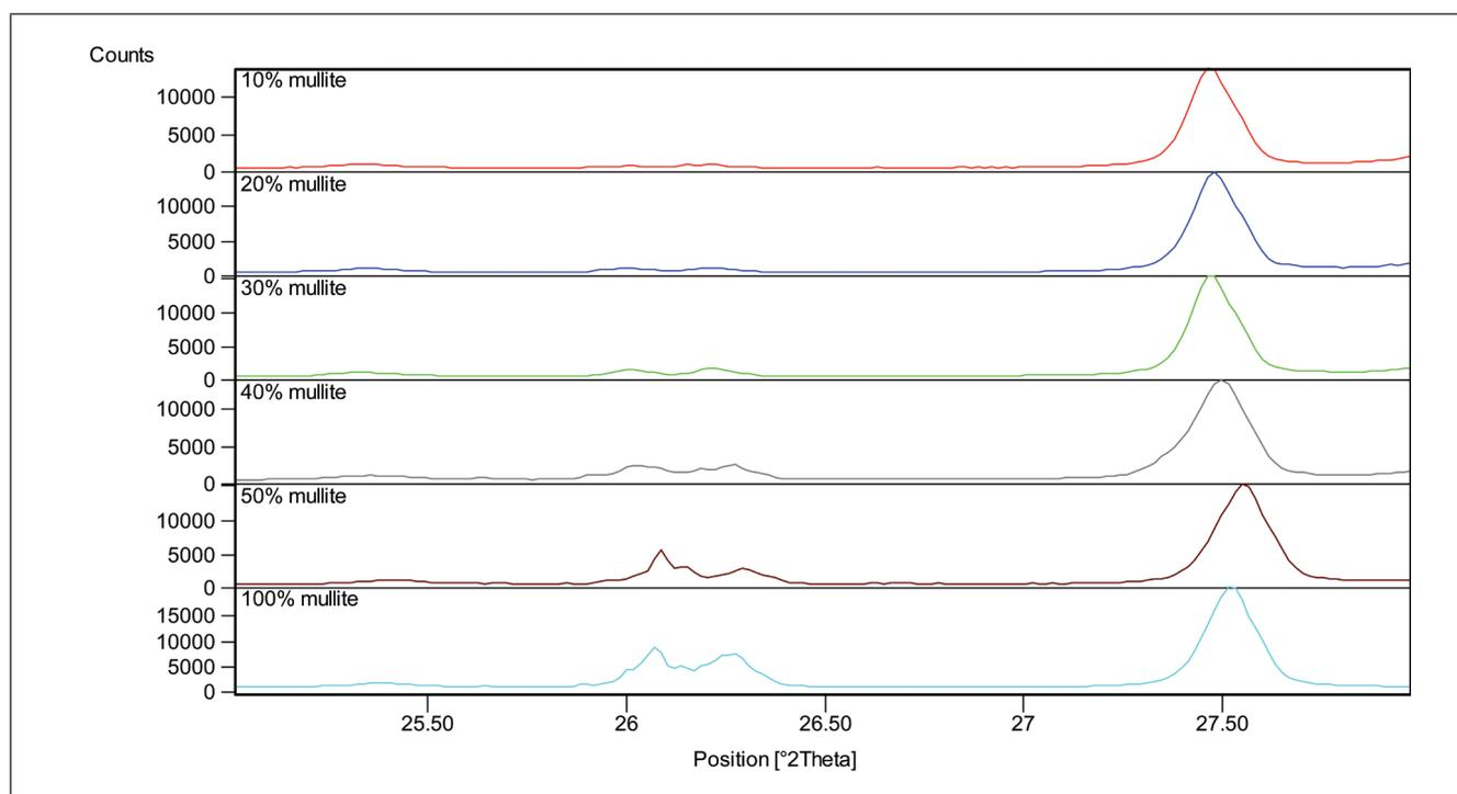
FIG. 4 X-RAY DIFFRACTION TRACES OF CALIBRATION RUNS FOR MULLITE ANALYSIS
