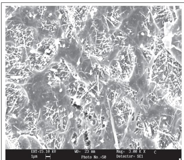
FIG. 2 ALUMINA BASED PORCELAIN INSULATOR WITH HIGH MULLITE CONTENT
