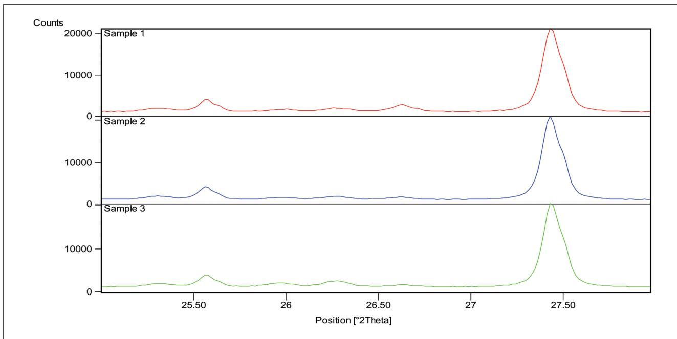
FIG. 6 VARIATION OF MULLITE IN ALUMINA BASED PORCELAIN INSULATORS SAMPLES
