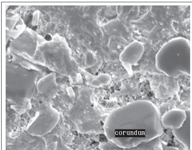
FIG. 1 ALUMINA BASED PORCELAIN INSULATOR WITH OPTIMUM MULLITE CONTENT
