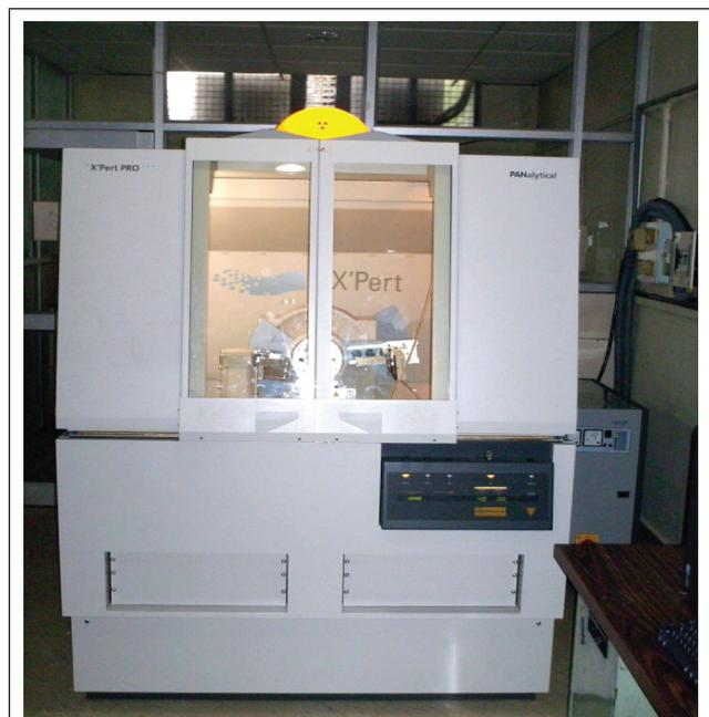
FIG. 3 X RAY DIFFRACTOMETER
