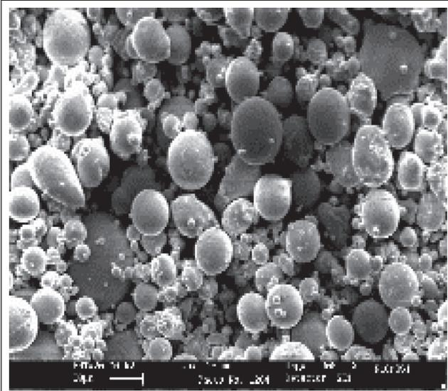
FIG. 2 SCANNING ELECTRON MICROGRAPH OF WC-CO/NICRBSI
