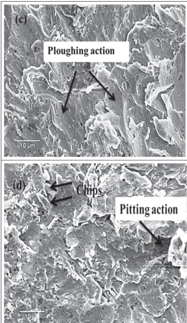
FIG. 9 SEM MICROGRAPHS SHOWING ERODED SURFACE MORPHOLOGY OF SS-310 STEEL AT 30° AND 90° IMPACT ANGLES. DIRECTION OF PARTICLE IMPINGMENT IS FROM TOP TO BOTTOM OF MICROGRAPHS. (A) AND (B) SHOWS SURFACE ERODED AT 25° C AND (C) & (D) SHOWS SURFACE ERODED AT 700° C.
