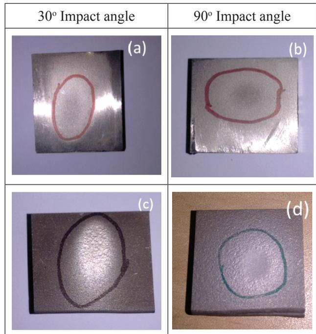
FIG. 5 CAMERA MACROGRAPH SHOWING THE EROSION SCAR AT 400° C PRODUCED ON THE SURFACE AT AN IMPACT ANGLE OF 30 DEG AND 90 DEG (NOT IN SCALE)(A) AND (B) UNCOATED STEEL (C) AND (D) WC-CO/NICRBSI
