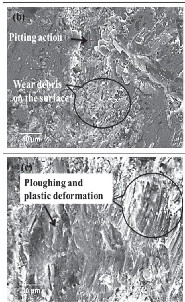
FIG. 10 SEM MICROGRAPHS SHOWING THE ERODED SURFACE MORPHOLOGY WC-CO-NICRBSI COATING AT 30° IMPACT ANGLES. DIRECTION OF PARTICLE IMPINGMENT IS FROM TOP TO BOTTOM OF MICROGRAPHS. (A) 25° C (B) 400° C AND (C) AT 700° C.
