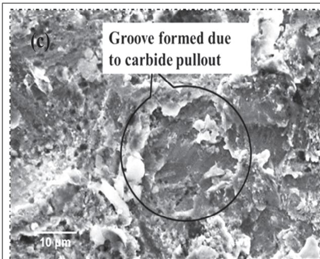
FIG. 11 SEM MICROGRAPHS SHOWING THE ERODED SURFACE MORPHOLOGY WC-CO/NICRBSI COATING AT 90° IMPACT ANGLES DIRECTION OF PARTICLE IMPINGMENT IS FROM TOP TO BOTTOM OF MICROGRAPHS. (A) 25° C (B) 400° C AND (C) AT 700° C.
