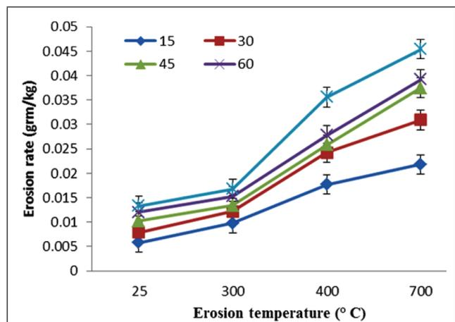
FIG. 6 THE EROSION RATE OF 35WC- CO/NICRBSI COATING WITH RESPECT TO THE EROSION TEMPERATURE AND IMPINGEMENT ANGLE.
