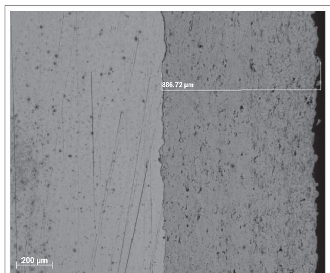
FIG. 4 THICKNESS OF COATING ON THE BASE PLATE
