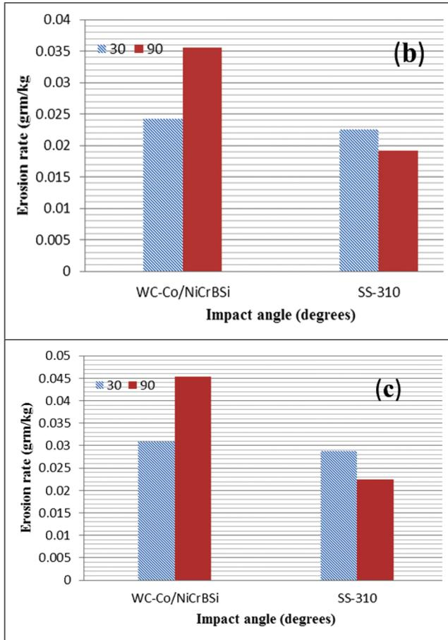
FIG. 7 HISTOGRAM ILLUSTRATING THE STEADY STATE EROSION RATE OF SS-310 (UNCOATED) AND WC-CO/NICRBSI COATED STEEL AT 30 AND 90 DEG IMPACT ANGLE FOR DIFFERENT TEMPERATURE RANGES (A) ROOM TEMPERATURE (25OC), (B) 400OC AND (C) 700OC TEMPERATURE.
