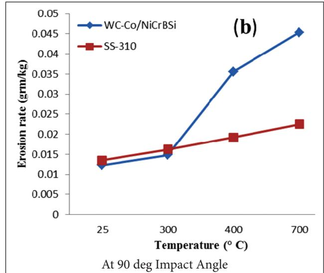
FIG. 8 VARIATION OF EROSION RATE WITH TEMPERATURE FOR WC-CO-NICRBSI AND SS-310 STEEL (A IMPINGMENT ANGLE OF 30O AND (B) IMPINGMENT ANGLE OF 90°, IMPINGEMENT VELOCITY 32 M/S.
