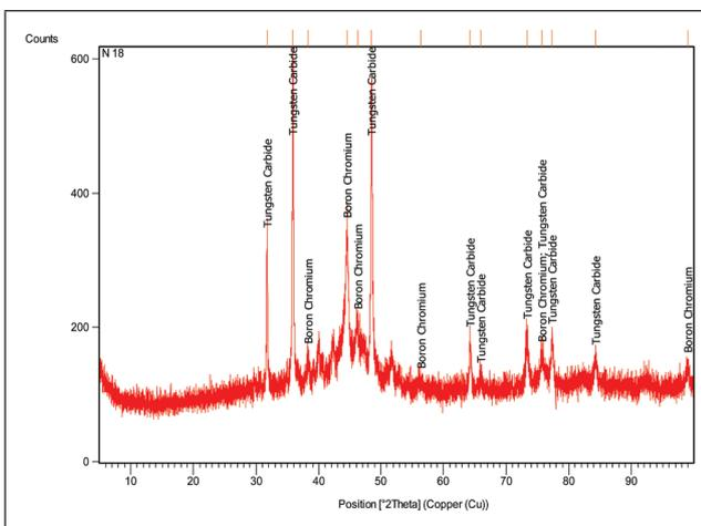
FIG. 3 X-RAY DIFFRACTION PATTERNS FOR POWDER
