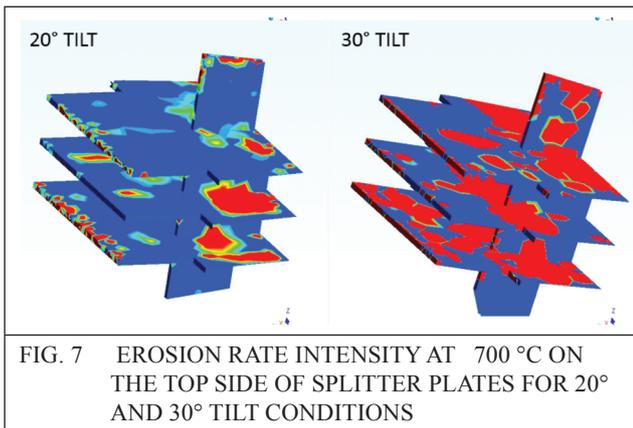
FIG. 7 EROSION RATE INTENSITY AT 700 °C ON THE TOP SIDE OF SPLITTER PLATES FOR 20° AND 30° TILT CONDITIONS
