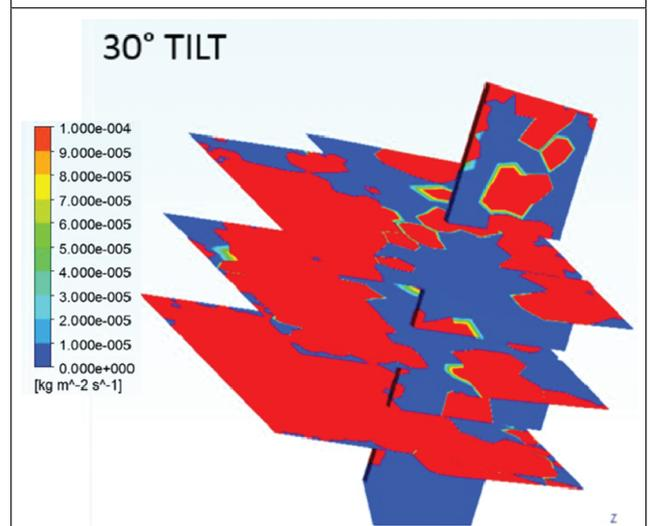
FIG. 6 EROSION RATE INTENSITY AT 700 °C ON THE BOTTOM SIDE OF SPLITTER PLATES FOR  $20^\circ$  AND  $30^\circ$  TILT CONDITIONS
