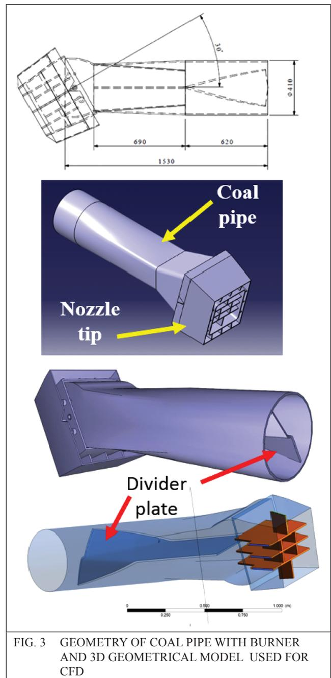
FIG. 3 GEOMETRY OF COAL PIPE WITH BURNER AND 3D GEOMETRICAL MODEL USED FOR CFD
