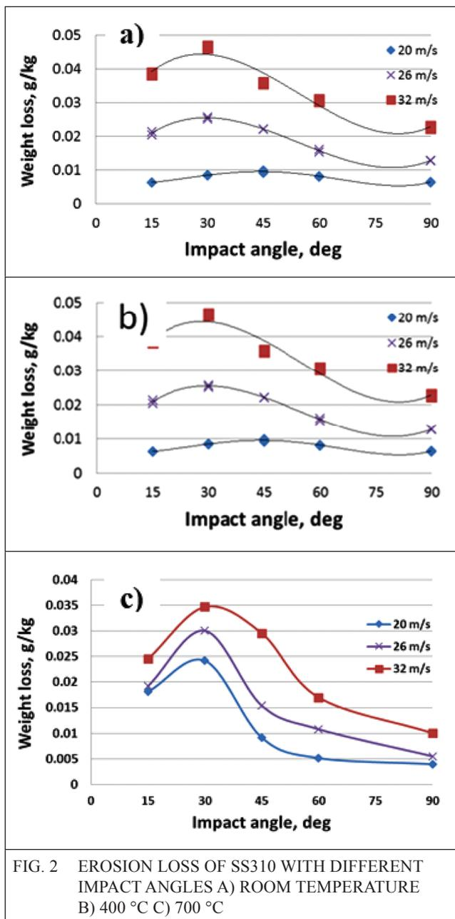
actual high-temperature erosion experiments conducted on the SS310 material. CFD approach is used to identify specific erosion regions in the coal burners with different tilt configurations of splitter plates. The particle erosion analysis process consists of a two-phase simulation of the transport of sand particles in the turbulent flow field where the impact of the particles on the components surface can be interactively monitored.
