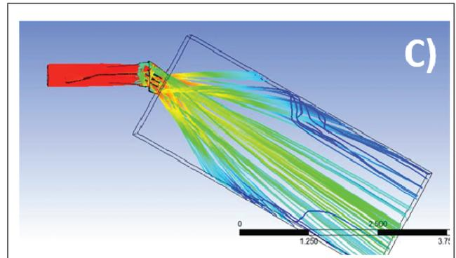
FIG. 5 PARTICLE TRACKING IN BURNER FOR DIFFERENT TILT CONDITION A)  $10^\circ$  B)  $20^\circ$  C)  $30^\circ$
