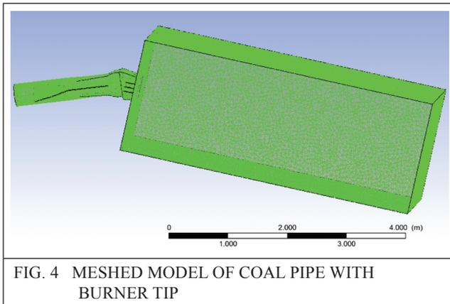
FIG. 4 MESHED MODEL OF COAL PIPE WITH BURNER TIP
