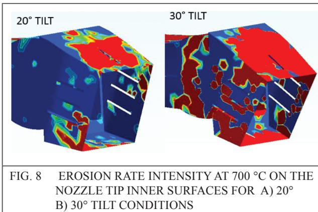
FIG. 8 EROSION RATE INTENSITY AT 700 °C ON THE NOZZLE TIP INNER SURFACES FOR A) 20° B) 30° TILT CONDITIONS
