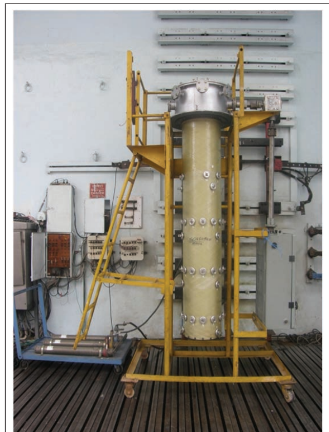
FIG. 13. MOUNTING ARRANGEMENT FOR SC TEST
