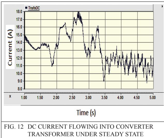
FIG. 12 DC CURRENT FLOWING INTO CONVERTER TRANSFORMER UNDER STEADY STATE
