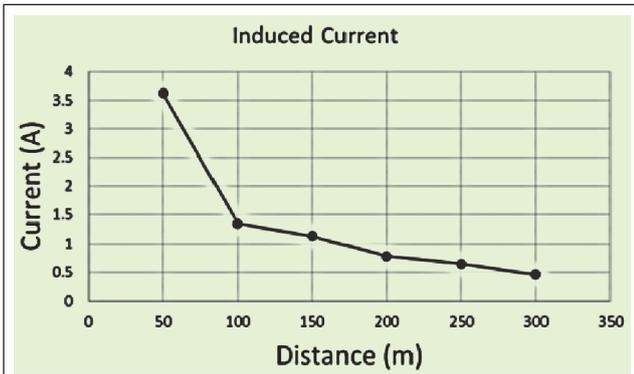
FIG. 8 MAGNITUDE OF INDUCED CURRENT UNDER LINE TO LINE FAULT
