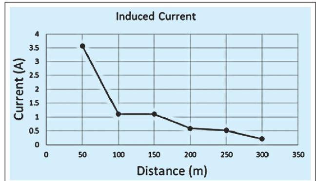
FIG. 6 DC CURRENT (A) FLOWING INTO THE CONVERTER TRANSFORMER AT STEADY STATE
