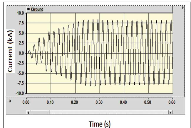
FIG. 11 CURRENT (A) IN THE EARTH SWITCH CONNECTED TO DC LINE
