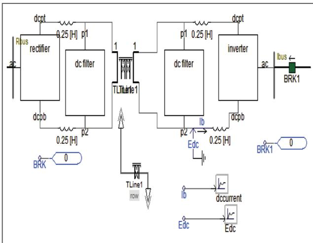
FIG. 1 DC SYSTEM MODELLED IN PSCAD™
