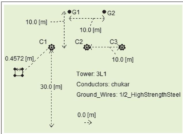
FIG. 2 DOUBLE CIRCUIT TRANSMISSION LINE IN PSCAD™
