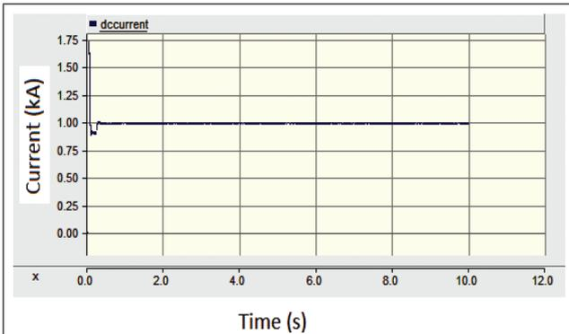
FIG. 4 STEADY STATE DC (kA) CURRENT
