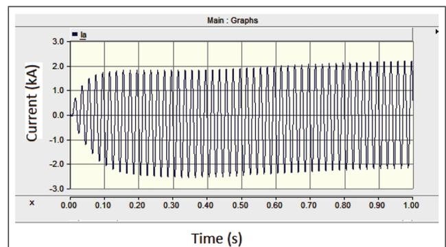
FIG. 3 STEADY STATE PHASE CURRENT (kA) IN AC LINE
