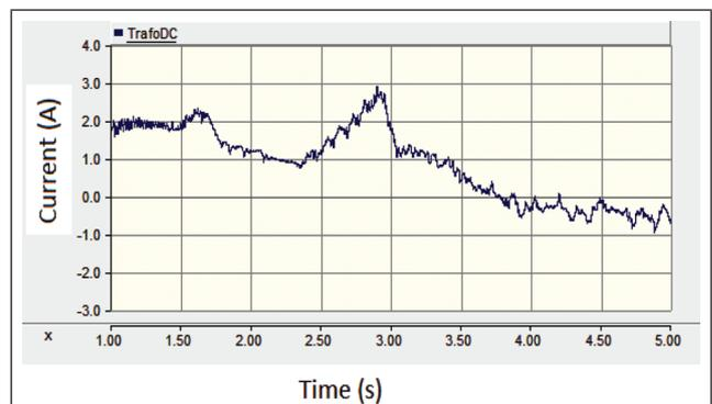
FIG. 7 MAGNITUDE OF INDUCED CURRENT UNDER THREE PHASE FAULT
