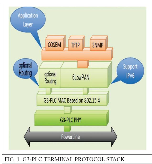
G3-PLC is an OFDM modulation based technology, which guarantees fast data transfer over existing power-lines within 150-500 kHz frequencies (CENELEC A band (within 35-91 kHz) or CENELEC B band (within 98-122 kHz) in Europe, on ARIB band (within 155-403 kHz) in Japan, FCC band (within 155-487 kHz) in USA and the rest of the globe is secure and stable
