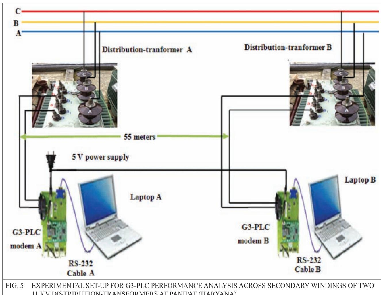
**FIG. 5 EXPERIMENTAL SET-UP FOR G3-PLC PERFORMANCE ANALYSIS ACROSS SECONDARY WINDINGS OF TWO 11 KV DISTRIBUTION-TRANSFORMERS AT PANIPAT (HARYANA)**
