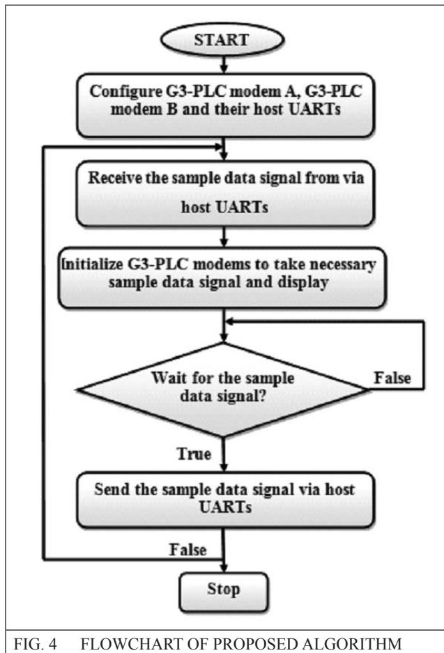
FIG. 4 FLOWCHART OF PROPOSED ALGORITHM
