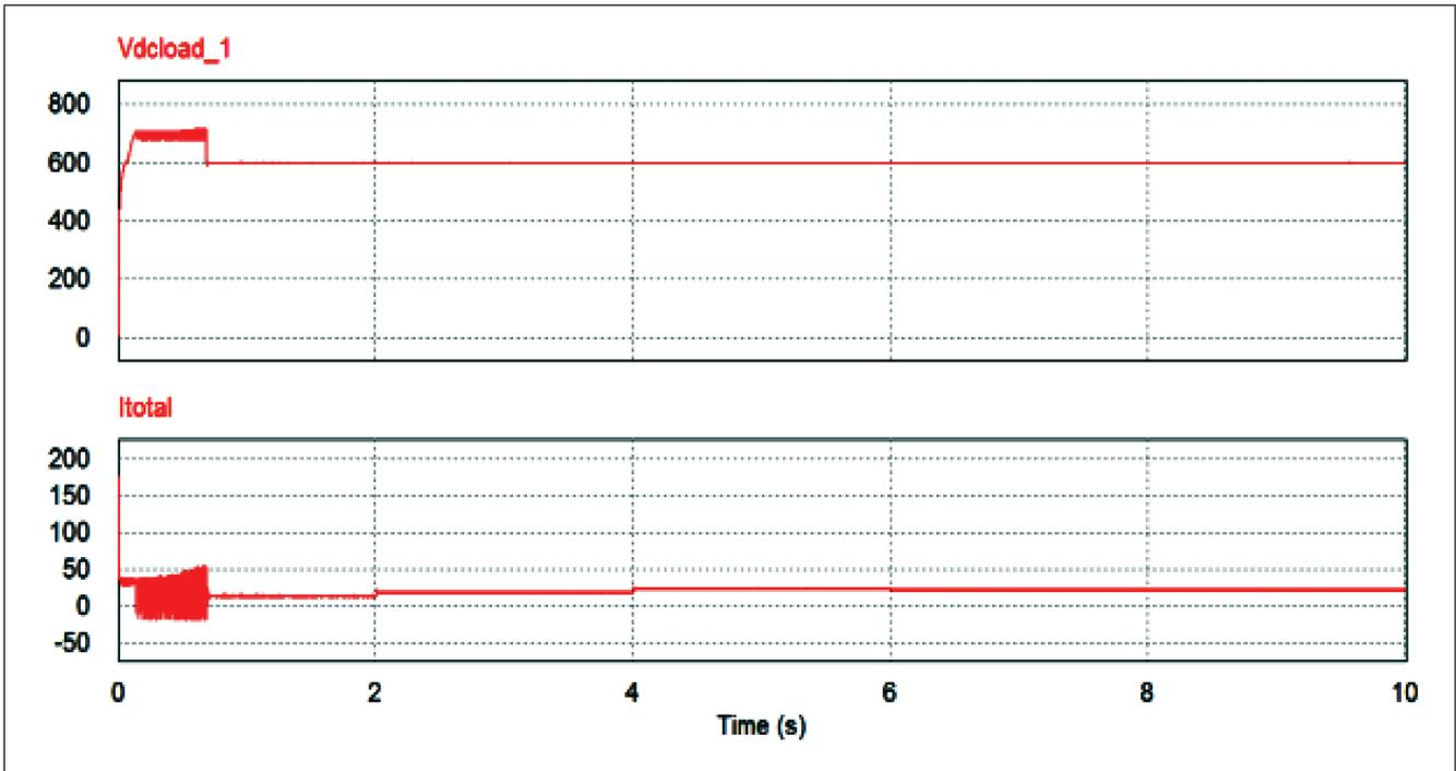
FIG. 3 DC LINK VOLTAGE AND TOTAL DIRECT CURRENT DRAWN BY SYSTEM.
