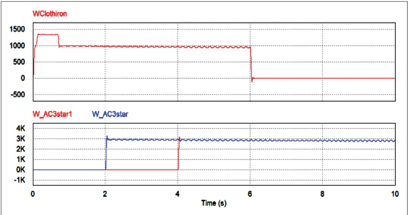
FIG. 5 SWITCHING OF LOADS (TWO NOS. OF THREE STAR AC AND CLOTH IRON)
