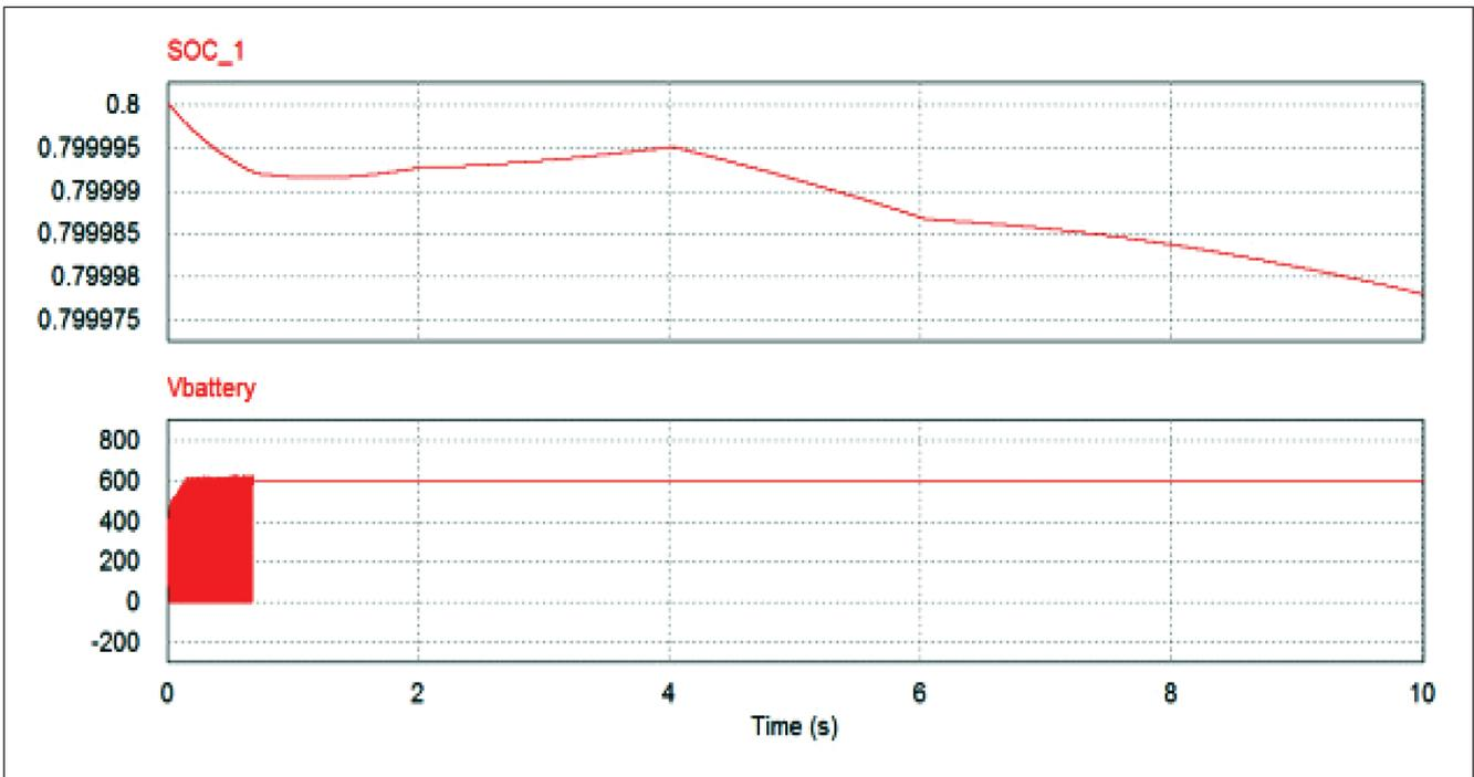
FIG. 8 STATE OF CHARGE OF BATTERY BANK AND VOLTAGE ACROSS DC BUS FROM BATTERY END.
