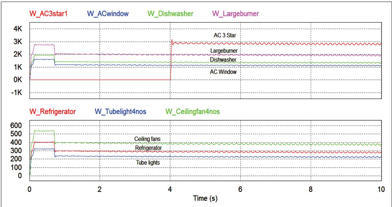
FIG. 4 POWER CONSUMED BY VARIOUS ELECTRICAL APPARATUS
