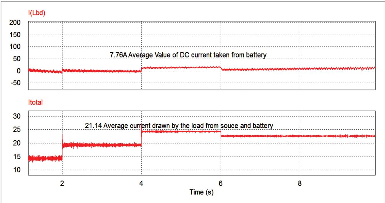
FIG. 6 CURRENT SHARED BY BATTERY AND TOTAL CURRENT DRAWN BY LOAD
