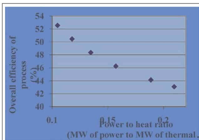
FIG. 6. OVERALL EFFICIENCY OF THE PROCESS (%).
