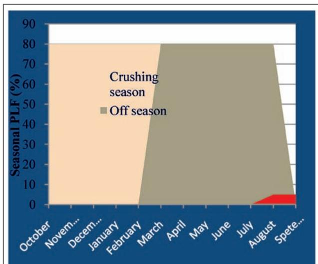
FIG. 10. TYPICAL SEASONAL PLANT LOAD FACTORS FOR THE CONVENTIONAL SUGAR BASED CHP PLANT WITHOUT CST.
