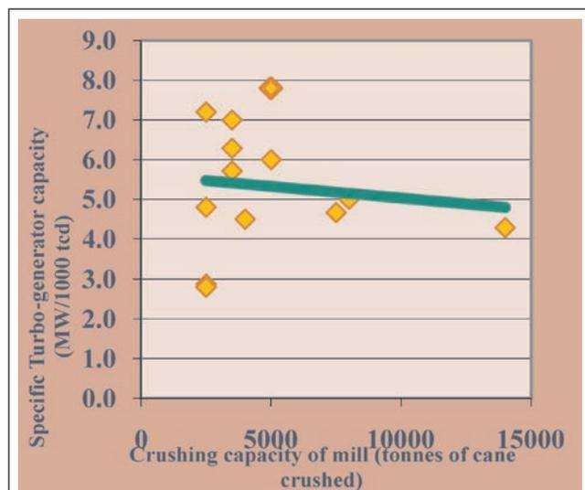
FIG. 5. TURBO-GENERATOR CAPACITY (MW) PER 1000 TONNES OF CANE CRUSHED
