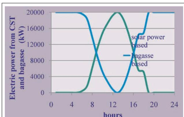
FIG. 9 POWER GENERATION PATTERN FROM CST PLANT WHEN INTEGRATED WITH SUGAR (BAGASSE FUELED) BASED PLANT.
