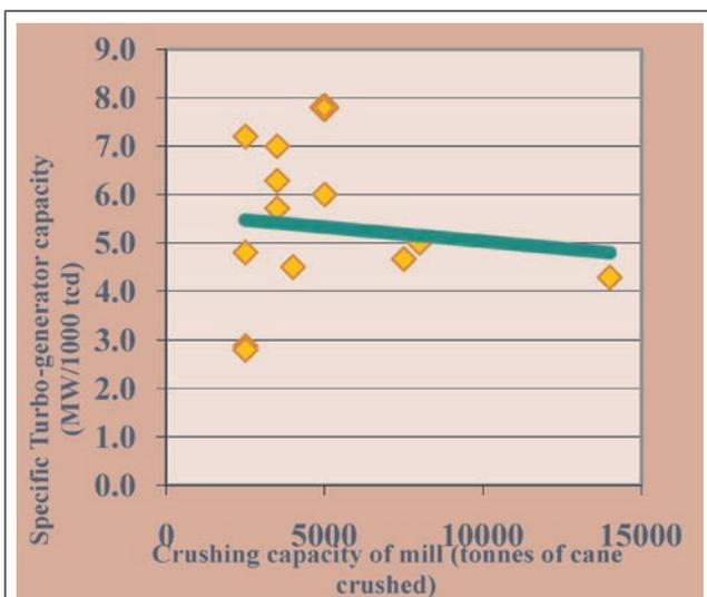
FIG. 5. TURBO-GENERATOR CAPACITY (MW) PER 1000 TONNES OF CANE CRUSHED
