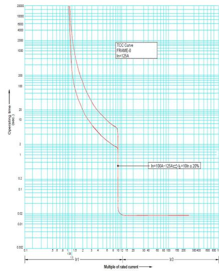
Figure 8. Time current characteristics for In = 125A (Frame-S).
