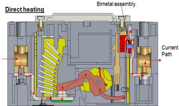
Figure 5. Cross sectional view for Direct Heating Method.
