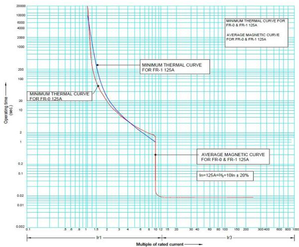
**Figure 3.** Thermal Magnetic TCC Curve for In = 125A (Frame-S & 1).
