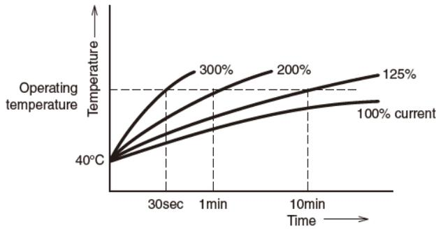
**Figure 2.** Deflection of bi-metallic strip as a function of Time and current<sup>3</sup>.
