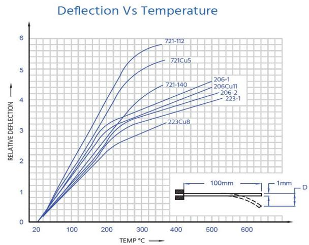
**Figure 4.** Relative deflection of bimetallic strip with respect to temperature.
