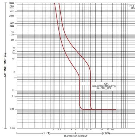
Figure 9. Time current characteristics for In = 125A (Frame-1).
