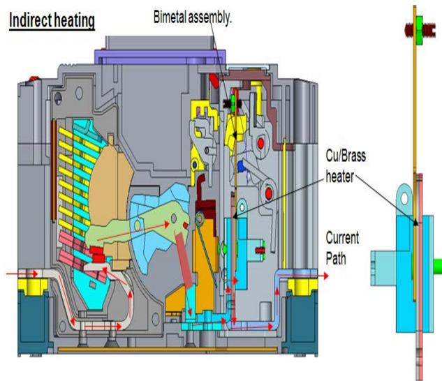
Figure 6. Cross sectional view for indirect heating.
