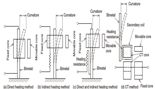
Figure 1. Different types of Bi-Metallic Heating Methods<sup>3</sup>.
