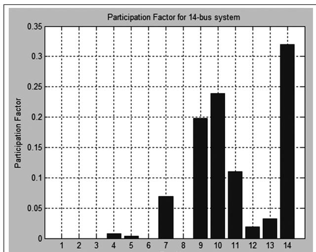
FIG. 9 BUS PARTICIPATION FACTOR ASSOCIATED FROM MINIMUM EIGENVALUE FOR CRITICAL OPERATING CASE.
