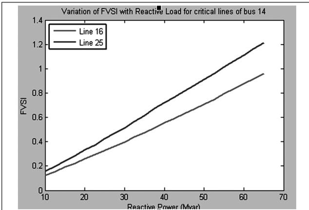
FIG.10 VARIATION OF FVSI WITH REACTIVE LOAD
