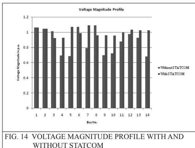
FIG. 14 VOLTAGE MAGNITUDE PROFILE WITH AND WITHOUT STATCOM
