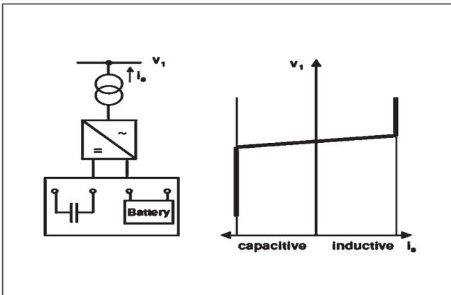
FIG. 5 STATCOM STRUCTURE AND VOLTAGE/ CURRENT CHARACTERISTIC
