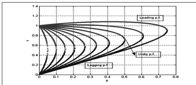
FIG. 1 TYPICAL P-V CURVE
