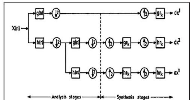
FIG. 3. SCHEMATIC REPRESENTATION OF IMPLEMENTATION OF MRSD.
