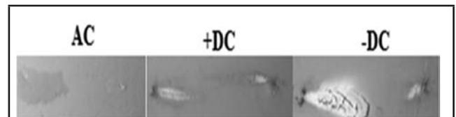
FIG. 5: SURFACE DAMAGE UNDER AC AND DC FIELD.
