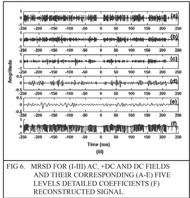
Figure 6 shows five level decomposition of the leakage currents under AC and DC voltages. Figure 7 shows STD\_MRA plot for the leakage current obtained during arcing under AC and DC fields. It is observed that high frequency content is high in leakage current measured under negative DC voltage as compared with the positive DC and AC voltage. Also it is observed that for AC fields the value of standard deviation is least and for negative DC field it is highest for all levels of decomposition.
