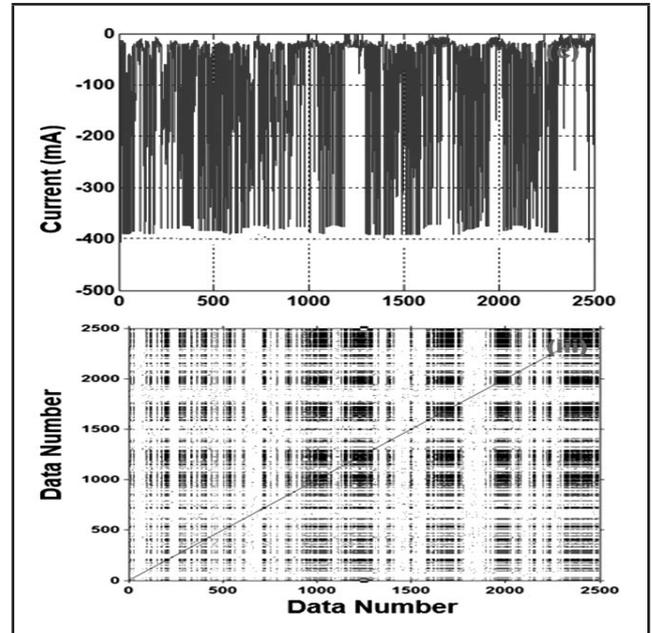
FIG. 4: LEAKAGE CURRENTS WAVESHAPES 4(A-C) UNDER AC, +DC AND -DC FIELDS AND THEIR CORRESPONDING RP 4(I-III)
