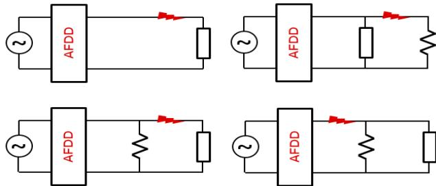
**Figure 4.** Test equipment for carbonized path tests.
