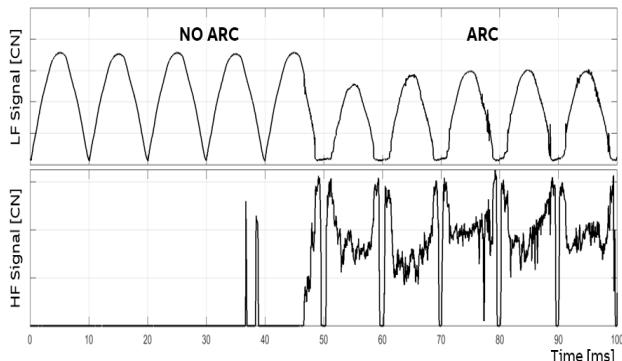
**Figure 9.** LF and HF signals seen by the MCU of an AFDD during a series arc carbonized path test.
