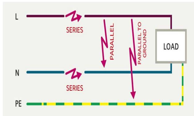
Figure 2. Classification of arc faults.
