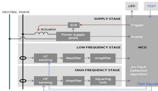
**Figure 8.** Functioning scheme of an AFDD printed circuit board.
