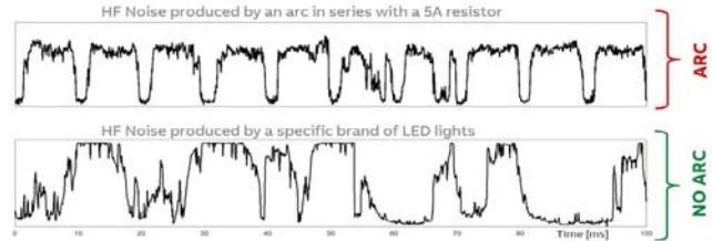
**Figure 11.** Comparison between the HF signal produced by an arc fault in series with a 5A resistor (above) and the HF signal produced by a specific brand of LED lights during normal functioning (below).
