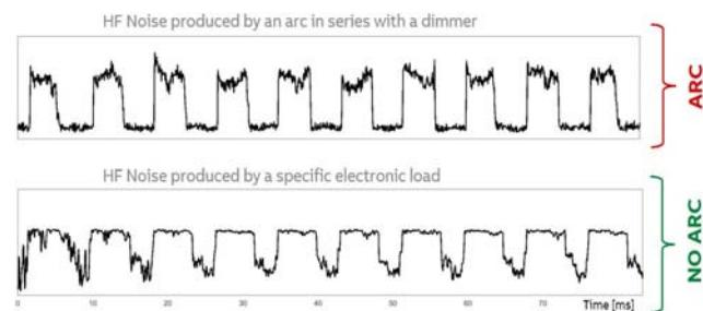
**Figure 12.** Comparison between the HF signal produced by an arc fault in series with a dimmer (above) and the HF signal produced by a specific electronic load during normal functioning (below).
