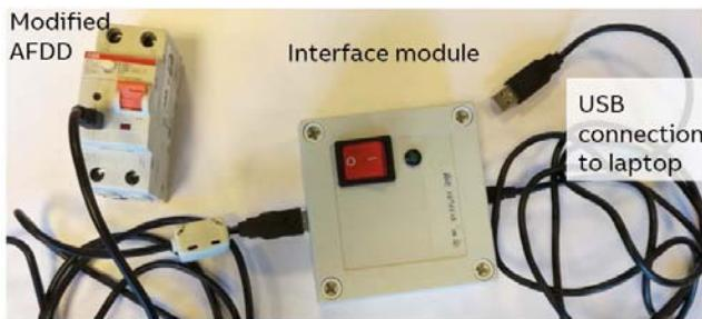
**Figure 14.** Modified AFDD breaker used to recorder data seen by the MCU during laboratory and field tests.
