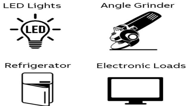
**Figure 10.** Examples of loads not foreseen by arc fault standards. Specific brands of these load my cause arc fault unwanted tripping.
