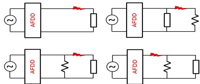
**Figure 5.** Configurations for carbonized path tests. The arc is created in a pre-carbonized sample of wire (in red). A resistor may be present together with a masking load (shown as a rectangle). Possible masking loads are listed in Figure 6.
