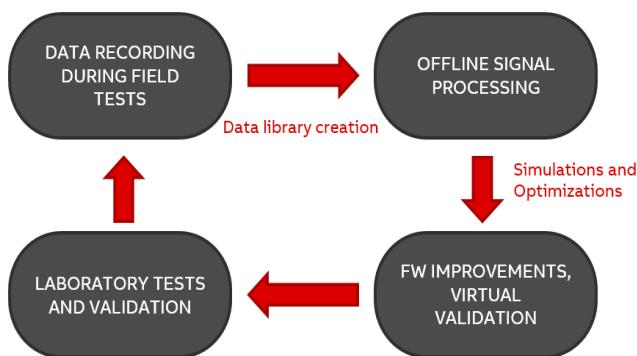
**Figure 13.** Method to improve arc fault detection algorithms.
