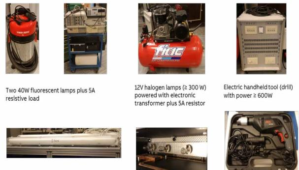
**Figure 6.** Masking loads in IEC62606.
