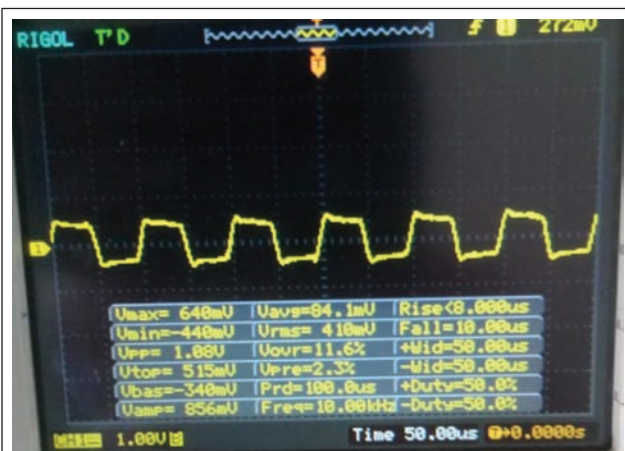
FIG. 6. SQUARED OUTPUT WITH HIGH SWITCHING FREQUENCY OF 10 KHZ SHOWN IN DIGITAL OSCILLOSCOPE
