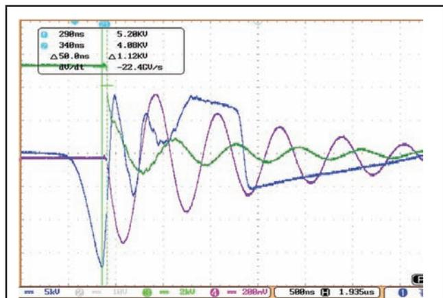
FIG. 5. DISCHARGE CURRENT (RED), NOT TO SCALE, CAPACITOR VOLTAGE (GREEN) AND TRIGGER VOLTAGE (BLUE) DURING ALL SEVEN CHANNEL DISCHARGE OF SEVEN CHANNEL SPARK GAP AT 5.5KV.
