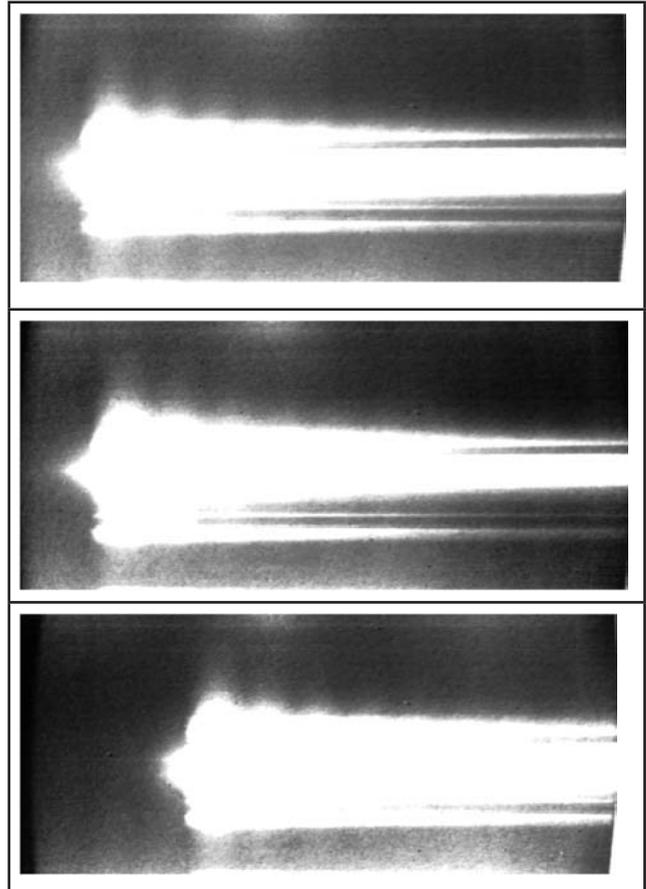
FIG. 4. STREAK IMAGES OF SEVEN CHANNEL SPARK GAP AT (A)4.0KV, (B)4.5KV, (C)5.0KV AND 5.5KV.
