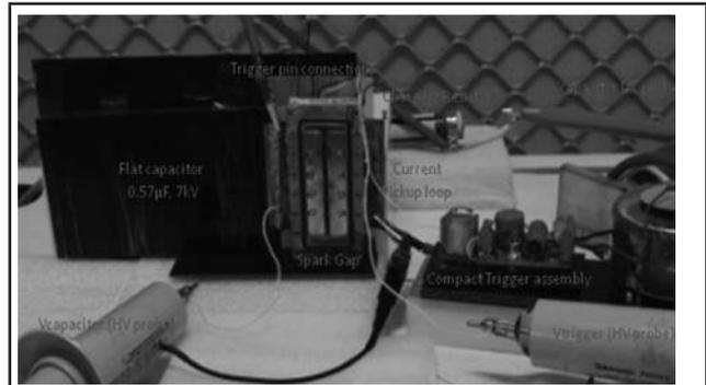
FIG 1. EXPERIMENTAL SETUP FOR MULTI CHANNEL SPARK GAP TESTING
