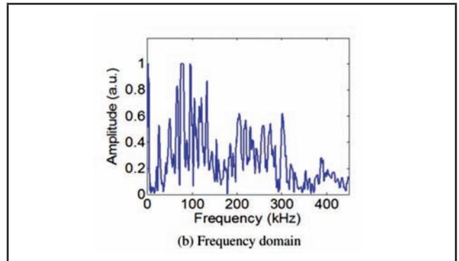
FIG. 2. SIGNALS CAPTURED BY FBG SENSOR FOR AN ELECTRODE GAP OF 1 CM IN BOTH (A) TIME AND (B) FREQUENCY DOMAINS
