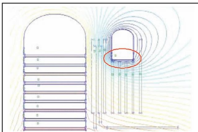
FIG 10 (A): WITHOUT SER FEM ANALYSIS- CRAWLING OF EQUIPOTENTIAL LINE NEAR EARTHED WINDING CORNER WITHOUT SER
