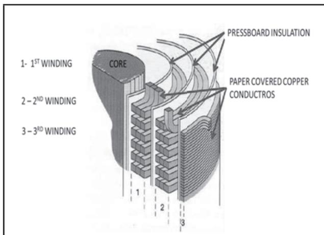
FIG. 1: CROSS SECTION OF THE CONCENTRICALLY ARRANGED CORE-WINDING ASSEMBLY WITH MIX INSULATION - PAPER, PRESSBOARD AND ALL SURROUNDED BY OIL [8]
