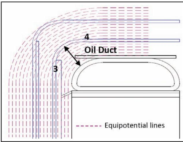
FIG 7 (B): CONTOURED ANGULAR WASHER
