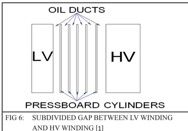
Table 2 shows the calculated maximum stress in each duct due to winding geometry, allowed stress for oil duct [9] and calculated safety factor for a small transformer with 29 mm HI-LO gap. Total HI-Lo gap is divided into 4 small oil ducts of 6 mm using 3 pressboard cylinders.
