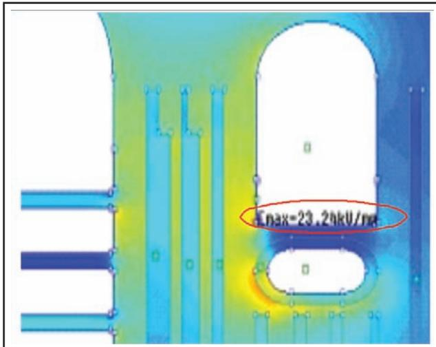
FIG 11 (B): WITH SER FEM ANALYSIS- REDUCED MAXIMUM FIELD STRENGTH TO 23.24KVP/ MM AT EARTHED WINDING CORNER
