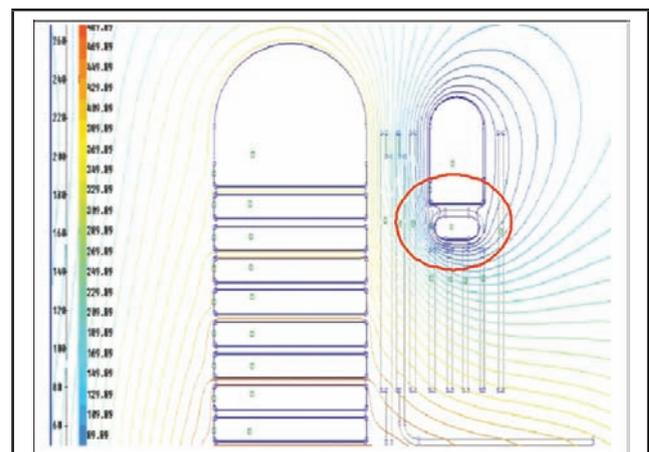
FIG 11 (A): WITH SER FEM ANALYSIS- SER REDUCES CONCENTRATION OF FIELD AT EARTHED WINDING CORNER
