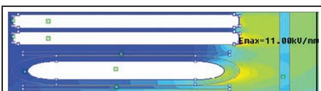
FIG 4: MAXIMUM ELECTRIC FIELD STRENGTH OBSERVED AT WINDIND CORNER WITHOUT 'L'- RING
