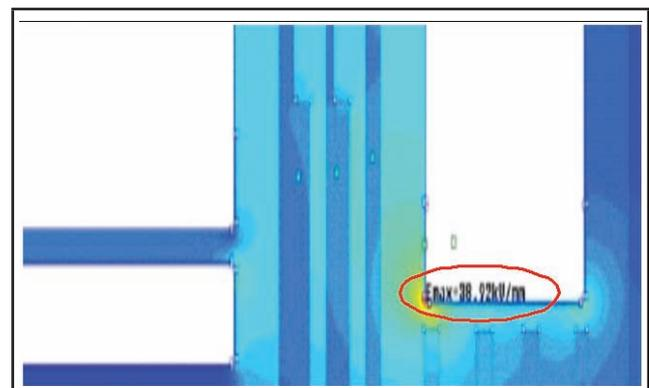
FIG 10 (B): WITHOUT SER FEM ANALYSIS- MAXIMUM FIELD STRENGTH OF 38.92 KVP/MM AT EARTHED WINDING CORNER WITHOUT SER
