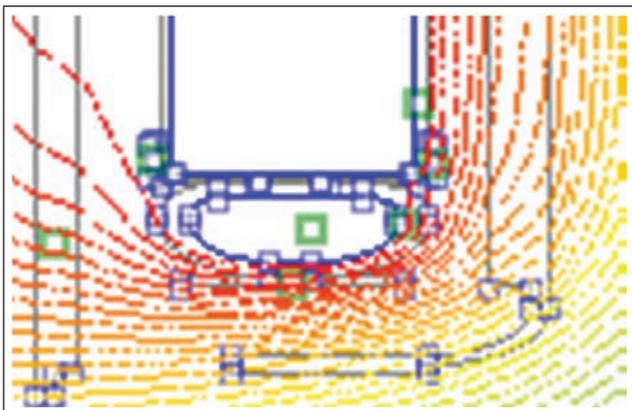
FIG 3: CRAWLING OF EQUIPOTENTIAL LINES NEAR END ZONE OF WINDING
