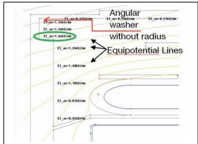
FIG. 8: NON CONTOURED ANGULAR WASHER
