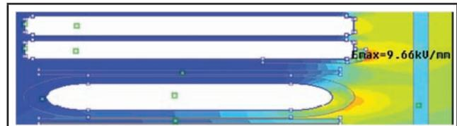
FIG 5: MAXIMUM ELECTRIC FIELD STRENGTH OBSERVED AT WINDING CORNER WITH 'L'- RING
