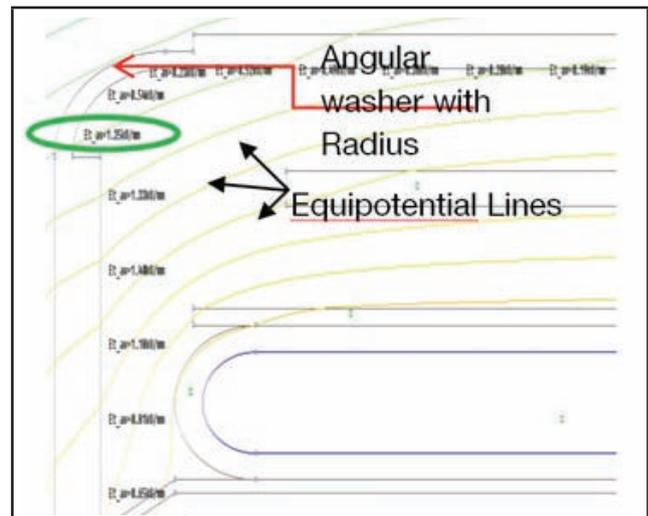
FIG 9: CONTOURED ANGULAR WASHER
