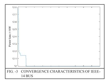
In 14 bus system also the population size, number of varying ORPD variables and maximum number of iterations were assumed suitably and the MAT lab programme was run.. This result and control variables are shown in Table-4. The loss values for 14-bus system of CBO algorithm compared with PSO, SARGA & MGBTL. It is observed that the loss minimization is improved by 1.21% from PSO, 2.03% from SARGA, 8.74% from MGBT and 11.04% from CBO algorithm.
