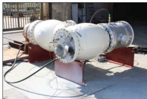
Figure 8. Test setup for clean air GIS [Courtesy Siemens Energy] (after test).
