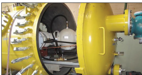
Figure 5. Test object (Single phase) inside test vessel (before test) [Courtesy Siemens Energy].
