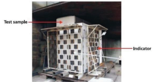
Figure 14. Internal arc test set up with indicators.
