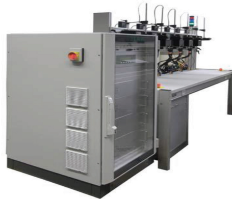
Figure 1. Six-position meter test system.
