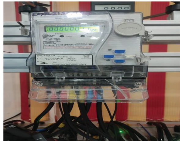
Figure 4. 3 phase 4 wire CT/PT operated smart energy meter.
