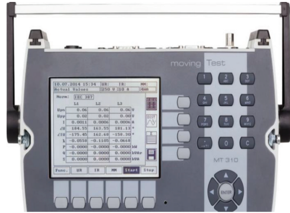
Figure 3. Portable reference meter for the experiment.
