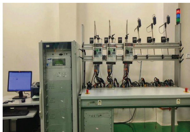
Figure 1. Test setup with 0.02% class reference meter.
