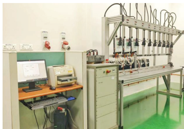
Figure 2. Test setup with 0.05% class reference meter.
