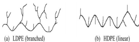
Figure 5. Structure of (a) LDPE (b) HDPE.
