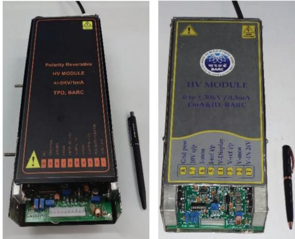
**Figure 10.** Polarity reversible 5kV/2mA and 30kV/0.3mA HV modules.
