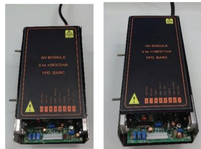
Figure 9. 5kV/2mA and 10kV/1mA HV modules.
