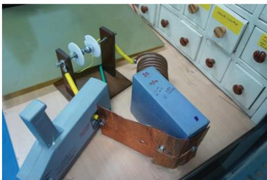
**Figure 4.** Setup for ESR measurement with one capacitor shorted.
