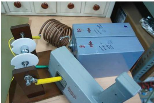
**Figure 3.** Setup for ESR measurement with both capacitor.
