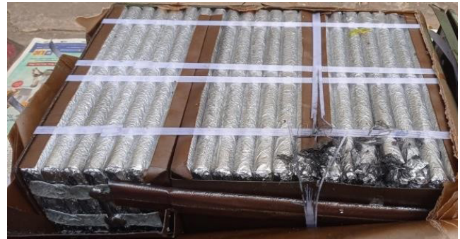
Figure 9. A view of the capacitor stack after removing from the capacitor container.
