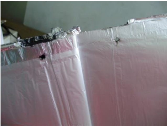
Figure 7. A view of puncture at edge of the element
