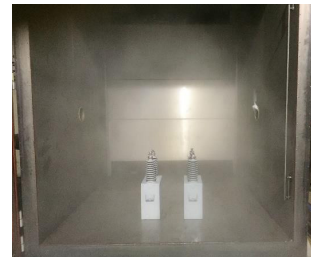
Figure 1. Arrangement for conditioning of capacitors in cold chamber at -40^\circ\text{C} .
