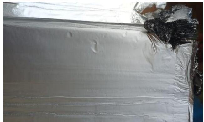
Figure 10. A view of the capacitor element indicating failure at the edge of the element.
