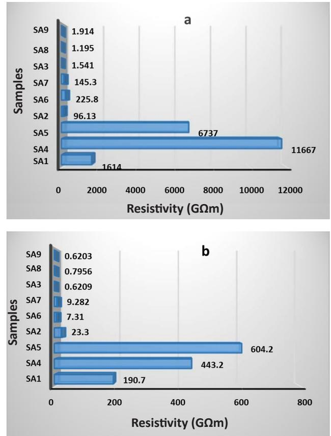
**Figure 5.** (a) Resistivity of samples, unaged. (b) Aged at 150 0C for 64 hours.
