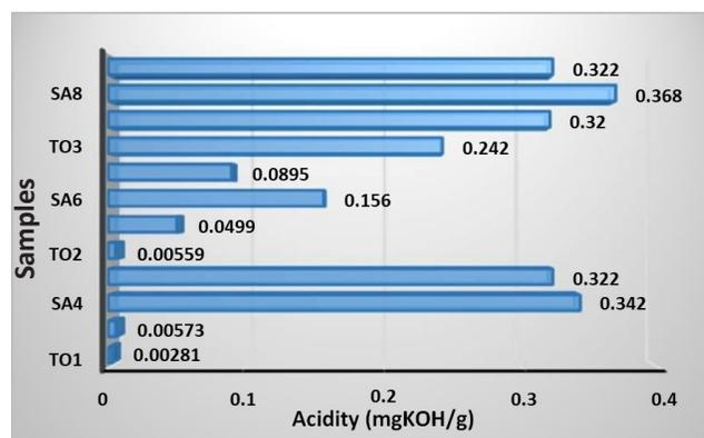
**Figure 3.** Acidity of samples, unaged (TO1, TO2, TO3), and aged at 150 0C for 64 hours (SA1 to SA9).
