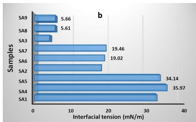
**Figure 2.** (a) Interfacial Tension (IFT) of samples, unaged. (b) Aged at 1500C for 64 hours.
