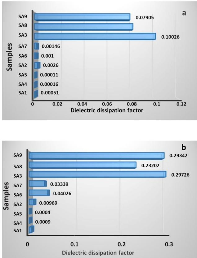
**Figure 4.** (a) Tan Delta of samples, unaged. (b) Aged at 1500C for 64 hours.
