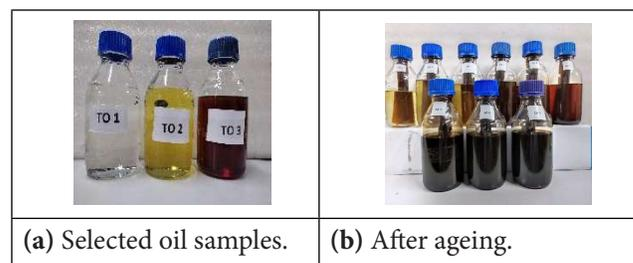
**Figure 1.** (a) Appearance of three oil samples taken for the study. (b) Nanofluids after laboratory thermal ageing.
