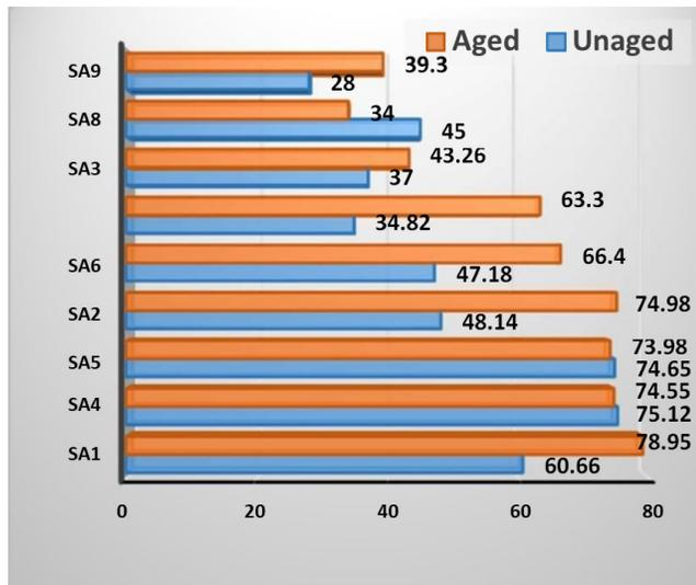
**Figure 6.** Breakdown voltage of unaged and samples aged at 150 °C for 64 hours.
