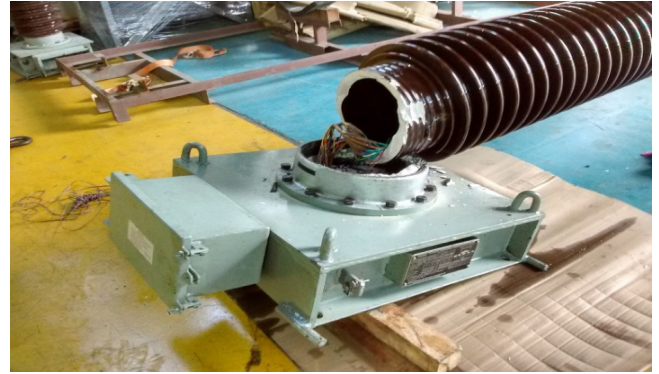
Figure 4. Close view of insulator after failure.
