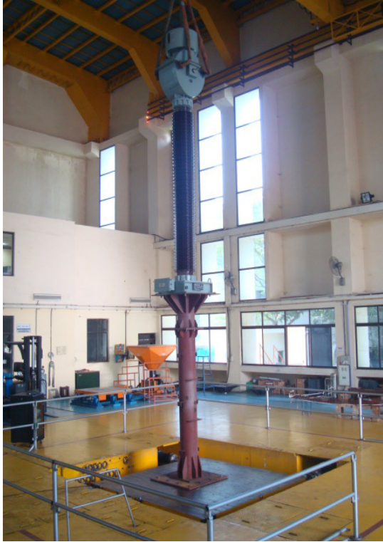
Figure 2. Live tank current transformer on shake table.
