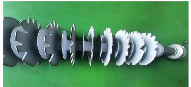
**Figure 7.** Deliberately damaged composite insulators like rodent/bird peaking damage.
