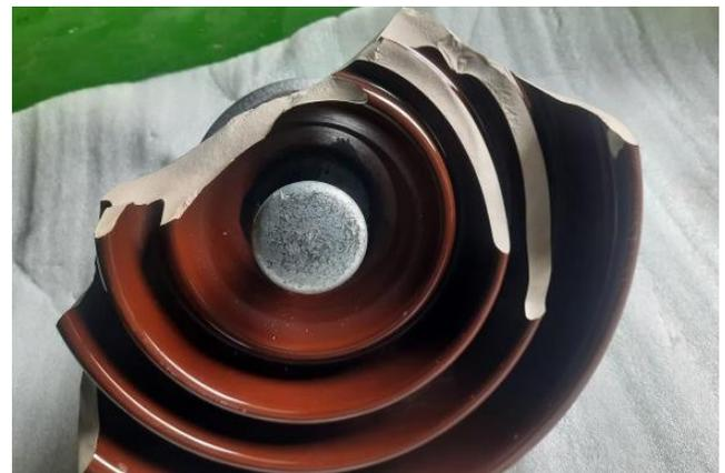
**Figure 8.** Deliberately damaged porcelain disc insulator.
