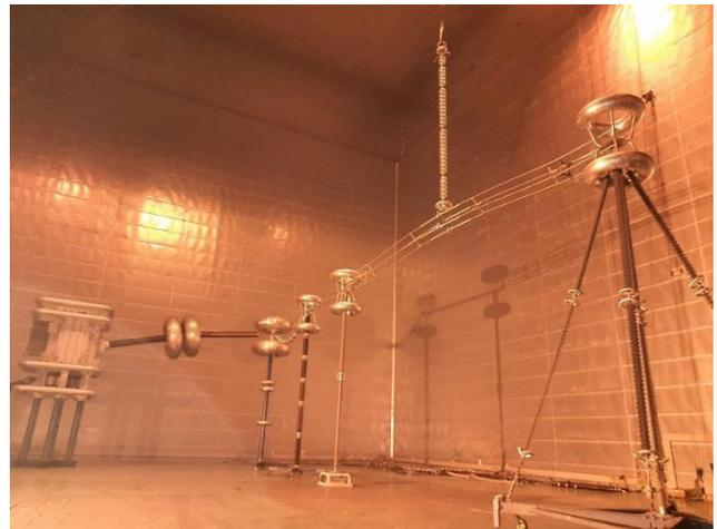
**Figure 1.** 765 kV glass disc insulator string with 5 damaged discs erected at double shielded indoor test facility for interference measurement.
