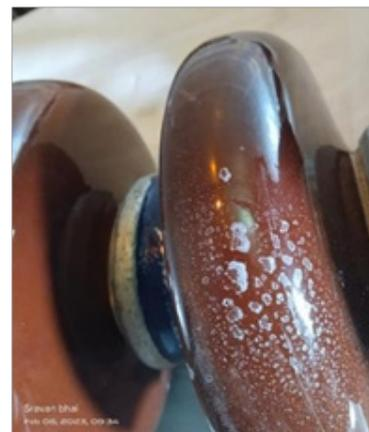
Figure 15. Porcelain disc insulator with salt water pollution applied on the surface.
