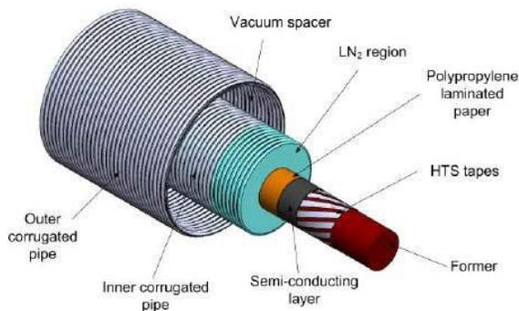
**Figure 1.** Schematic of single phase HTS power cable.
