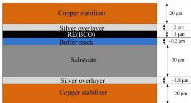
**Figure 2.** Schematic and thickness of different layers of an HTS tape.
