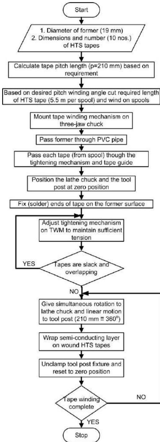
Figure 7. Flow chart for tape winding procedure.
