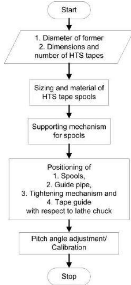
Figure 4. Flowchart for designing tape winding mechanism.
