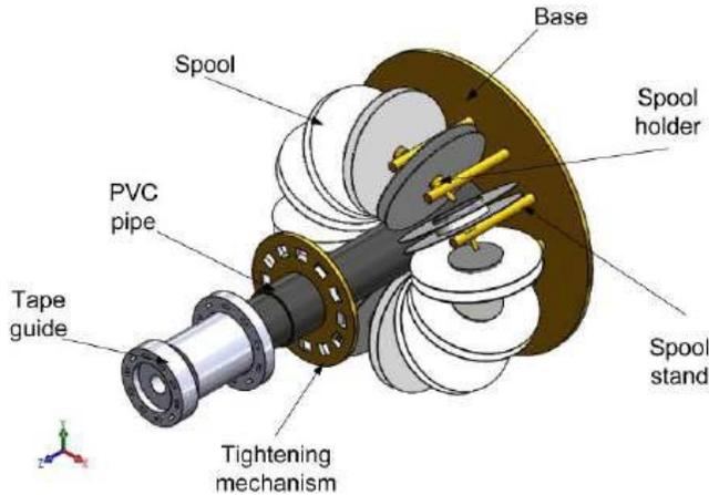
**Figure 5.** 3-D CAD model of spool holder and guide.
