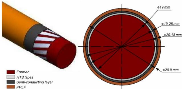
Figure 3. HTS cable core layers and dimensions.
