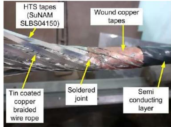
Figure 8. Photograph of the soldered joint to join HTS and copper tapes.
