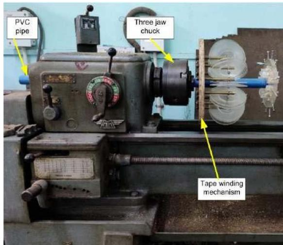
**Figure 6.** Photograph of lathe machine and tape winding mechanism.
