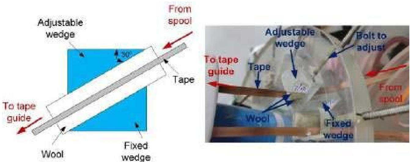
Figure 11. Cross-sectional view and photograph of the tightening mechanism.
