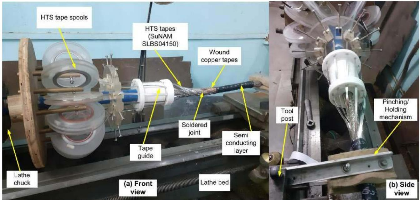
Figure 10. Photograph of front and side view of cable core during winding.
