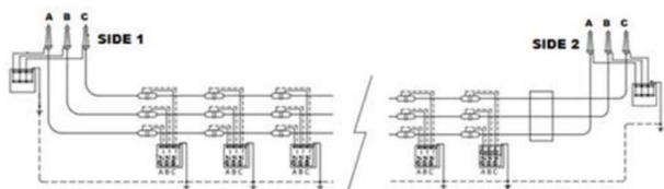
**Figure 9.** Schematic of a 3-phase 230 kV, 16.1 km long cable installation. Side 1 was used to inject the high voltage.
