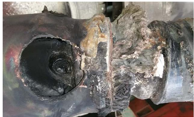
(e) Corroded shield.
