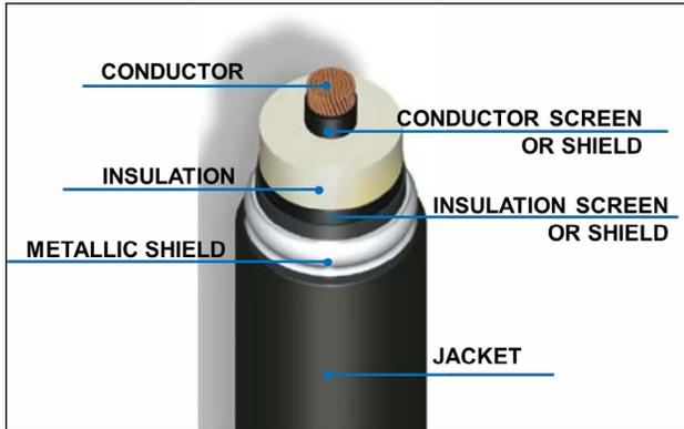
(a) Typical cable cross-section.
