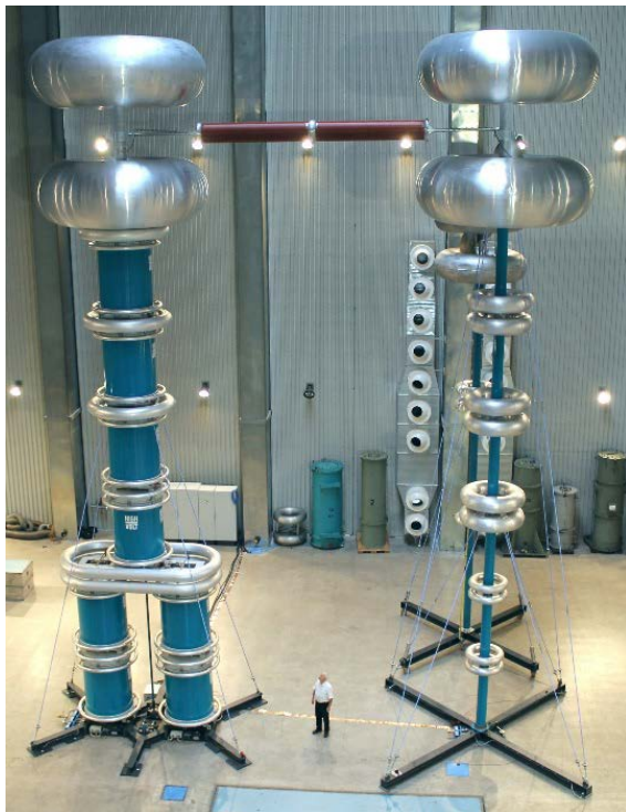
Figure 7. GPM 10/2200: 10 mA rated current and 2200 kV output voltage.
