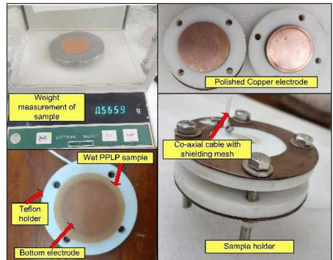
**Figure 9.** Photograph of weighing and positioning of PPLP sample.
