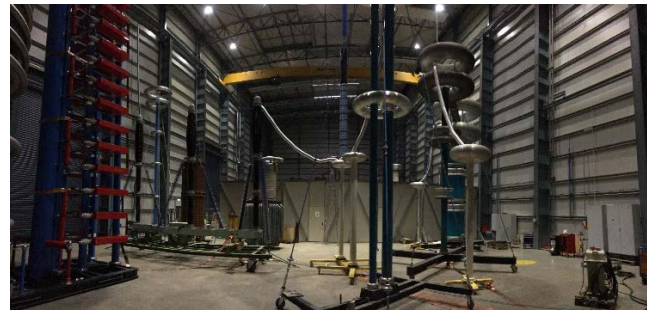
Figure 8. Example of a Laboratory set-up for the zero-crossing damped oscillatory discharge test.
