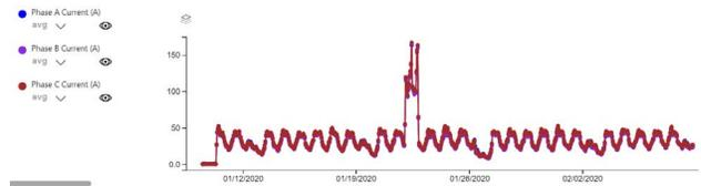
**Figure 8.** Source: Load curve plotted using 3MTM Sensored Cable Termination and Electrical Analytics Unit (EAU), a component of the 3M™ Underground Monitoring, Analytics and Communication System, with hourly time span for three core cable termination installed in ring-main-unit
