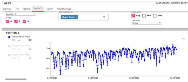
**Figure 6.** Source: Phase angle plotted using 3M™ Sensor Termination and 3M™ Underground Monitoring, Analytics and Communication System with hourly time installed in ring-main-unit at TPDDL.
