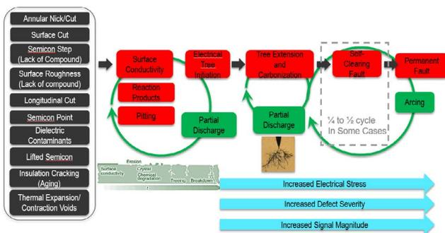
Figure 10. Life-cycle of Fault in Underground Cable Network<sup>5</sup>
