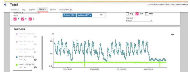
Figure 5. Source: Voltage and Current curve plotted using 3M Sensor Termination and 3M™ Underground Monitoring, Analytics and Communication System with hourly time installed in ring-main-unit at TPDDL.
