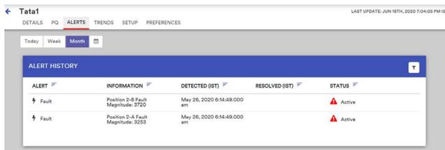
**Figure 7.** Source: Fault magnitude and alert captured using 3M™ Sensored Cable Termination and 3M™ Underground Monitoring, Analytics and Communication System installed in ring-main-unit at TPDDL.
