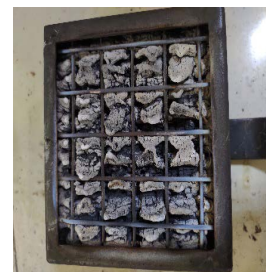
Figure 4. Cables in the sample holder before and after burning.
