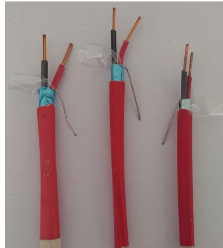
Figure 2. Fire Resistant cables with silicone insulation.
