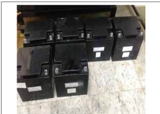
FIG. 3. HYBRID ULTRACAPACITOR OF 12V/2500F RANGE EMPLOYED FOR THE STUDY
