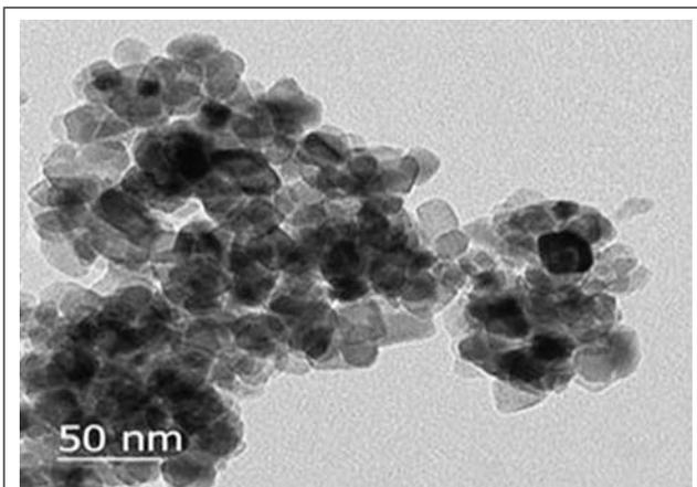
FIG. 1 TEM IMAGE OF  $\text{TiO}_2$  NANOPOWDER (50NM)
