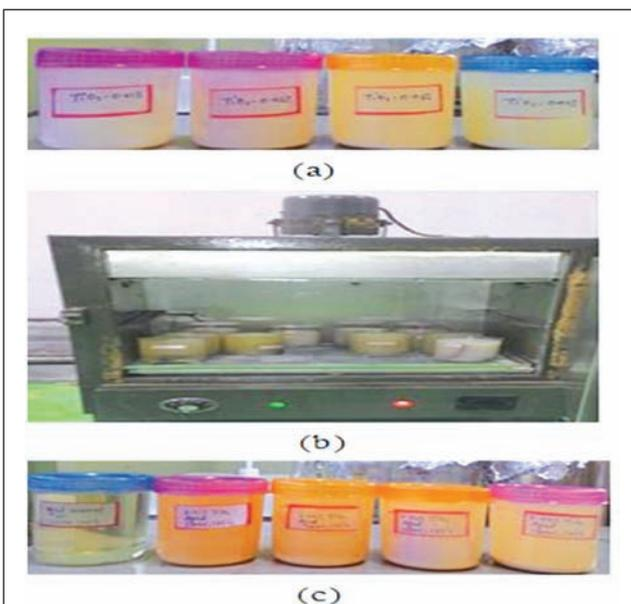
FIG. 2 (A) PREPARED SAMPLES OF NEW MINERAL OIL BASED  $\text{TiO}_2$  NANOFLUIDS; (B) ACCELERATED AGEING SAMPLES IN AGEING OVEN; (C) AGED SAMPLES OF  $\text{TiO}_2$  NANOFLUIDS
