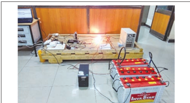
FIG. 12 UPS/INVERTOR AS LOADS TO POWERLINE COMMUNICATIONS
