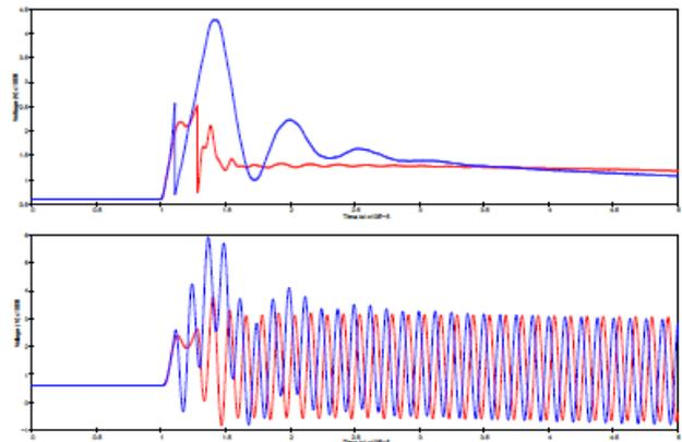
**Figure 5.** Voltage at substation entrance and transformer terminal (Blue graph is without arrester and Red graph is with arrester).
