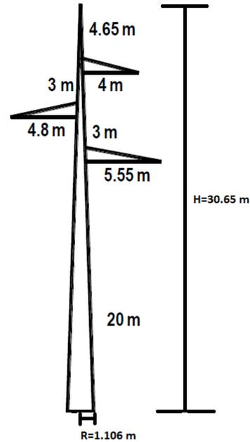
**Figure 2.** Transmission line geometry.
