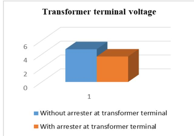
Figure 8. Comparison of transformer terminal voltage.
