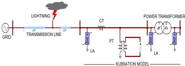
**Figure 1.** Single line diagram of the system considered.
