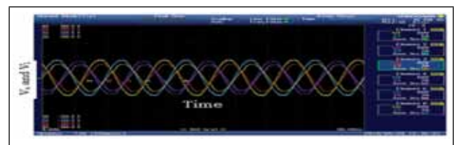
FIG.6 SOURCE AND LOAD VOLTAGE WITHOUT DSTATCOM
