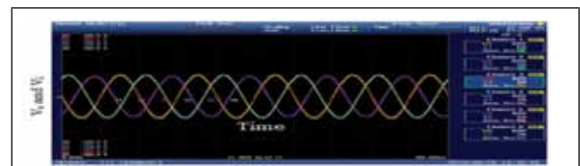
FIG.7 SOURCE AND LOAD VOLTAGE WITH DSTATCOM
