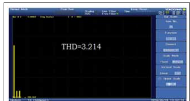
FIG.8 THD WITHOUT DSTATCOM
